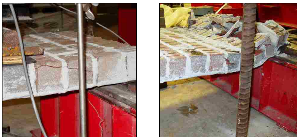
(a) Flexural-Shear Cracking
