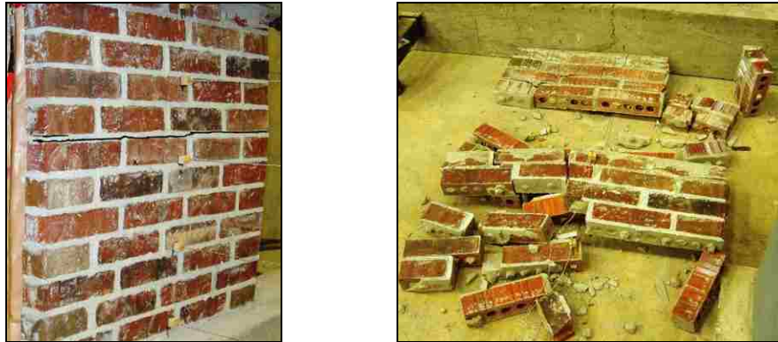
(a) Horizontal Crack
