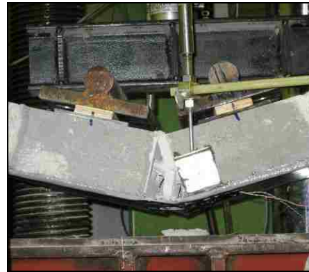
(b) Growth of Crack Width
