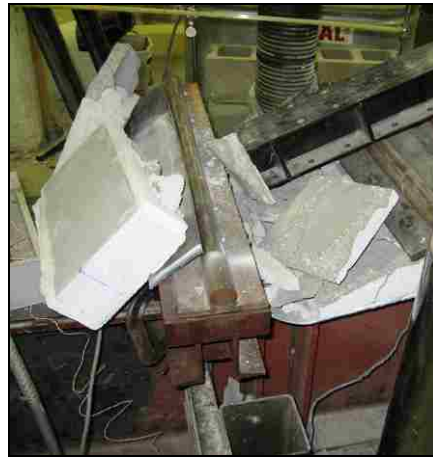
(b) Debonding of Masonry
