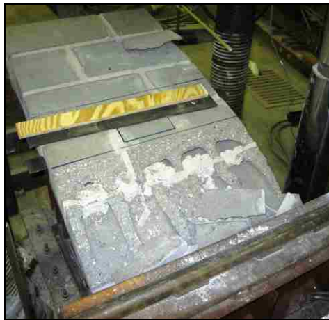
(c) Fracturing of Masonry
