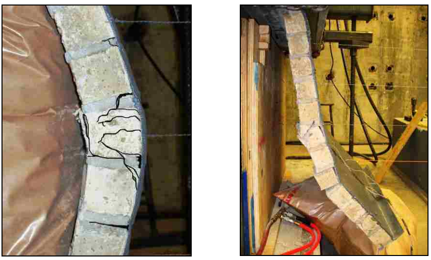
(b) Flexural Cracks in WF-FA
