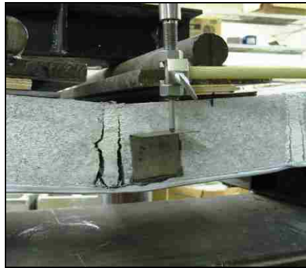
(a) Midspan Cracking
