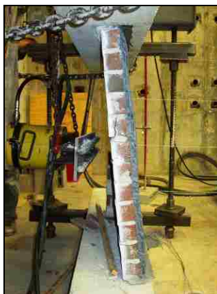
(c) Wall Failure
