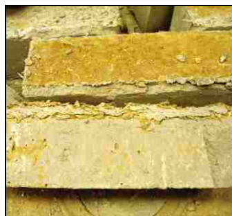
(c) Crushing of WF-FA Brick Units
